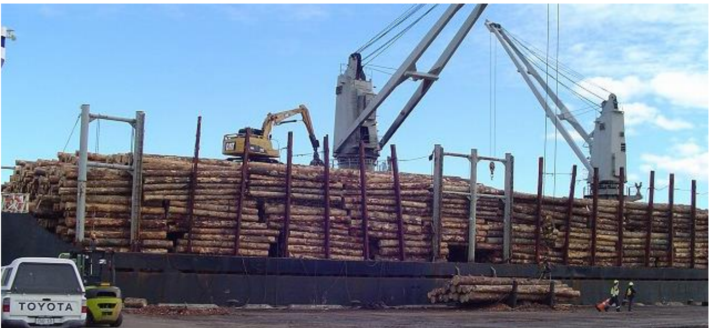
General view of a vessel loading logs on deck. Note the “bunk” alongside and the digger on deck. Just above the bunk we can see a gap in the stow in way of the permanent stanchions. This was left to give crew access to sounding pipes and ballast valves at the ship’s side, and to allow access for the fumigators to reach the hold manholes, to insert the phosphine blankets, just prior to sailing. Also, the top of the stow on deck is slightly “crowned”, to ensure that overlashings touch approx. 80% of the logs. This makes the lashing more effective and secure.
