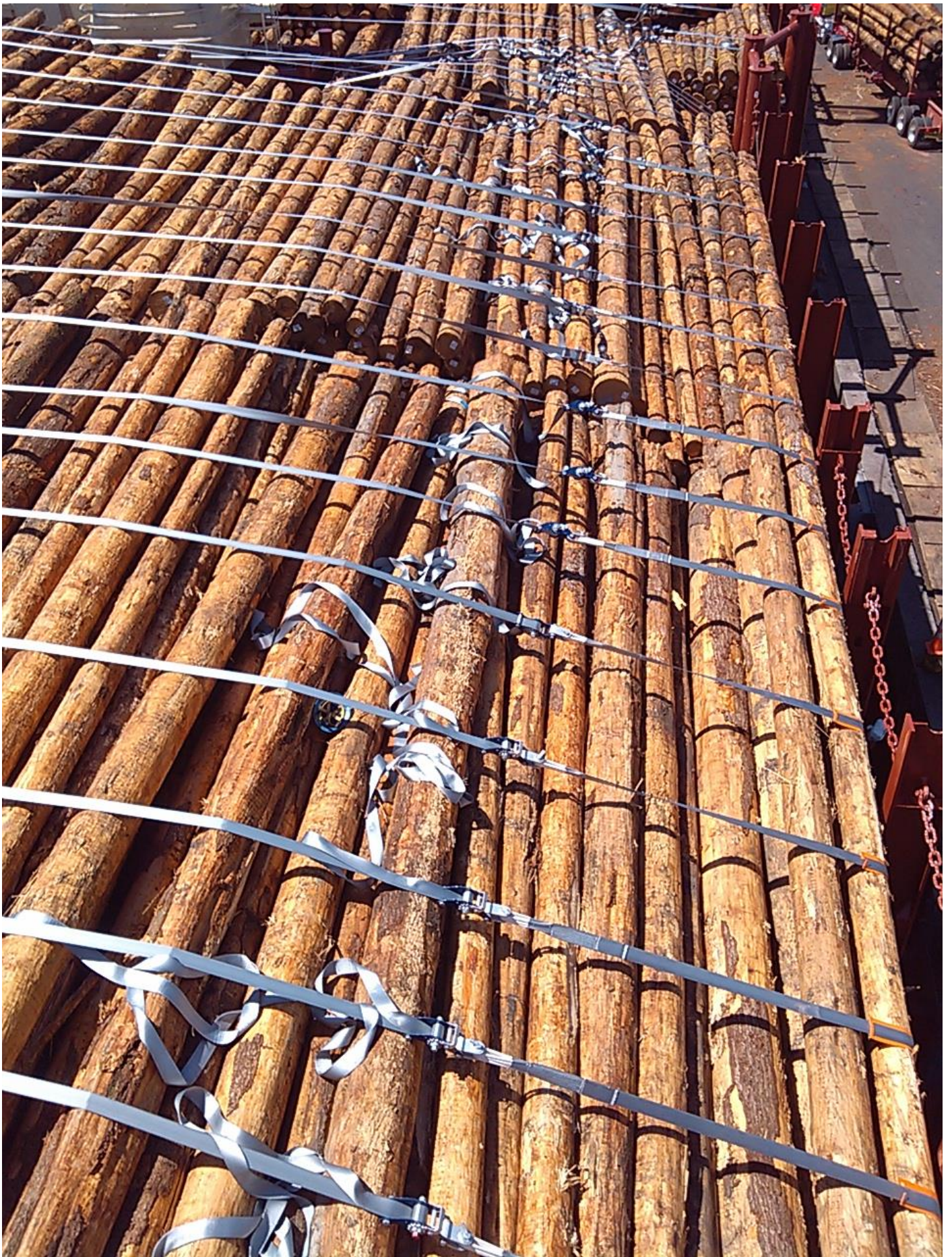
Another view of the vessel lashed with fibre lashings.
