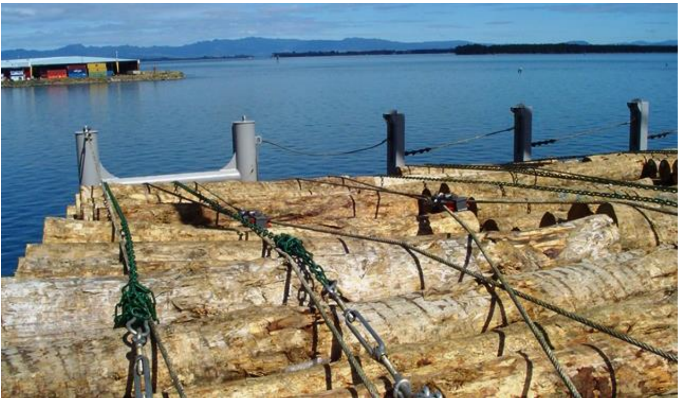
A closer view of a vessel lashed with individual chains and a “wobble wire” system.
