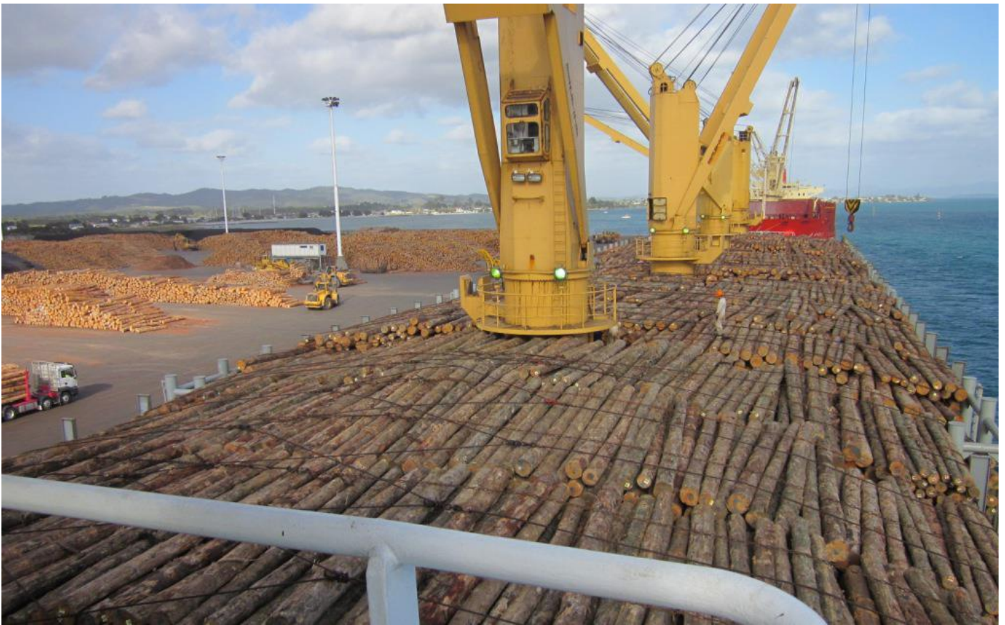
Completed vessel, fully lashed with a conventional lashing system, consisting of individual chains every 3 metres and a “wobble wire” system.
