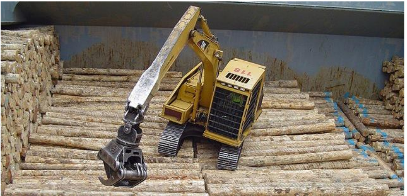
Typical “digger machine”, usually around 15-17 tonnes, with a rotating grapple attachment for handling the logs individually, or in packets of 2-4 pieces.
