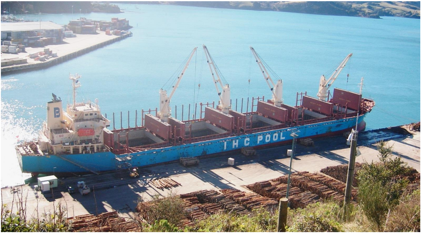
Typical Handysize vessel of about 28,500 dwt loading logs at Port Chalmers, New Zealand
