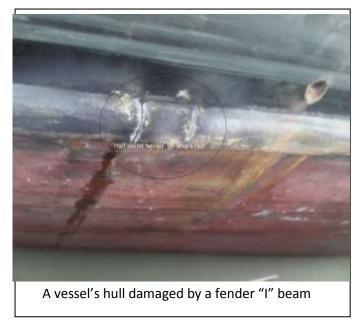
Mariners are advised to note the condition of the fenders and to take appropriate action during berthing and when alongside the pier. In the latter case tending/slackening mooring line may be needed to ensure that the hull is not pressed too tightly against the fender beams when there is a risk.
