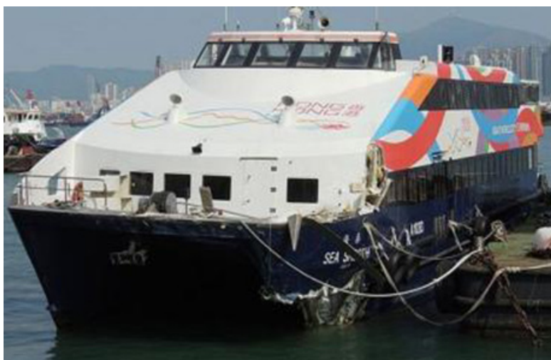
Sea Smooth was able to continue with bow damage and safely disembark her passengers
